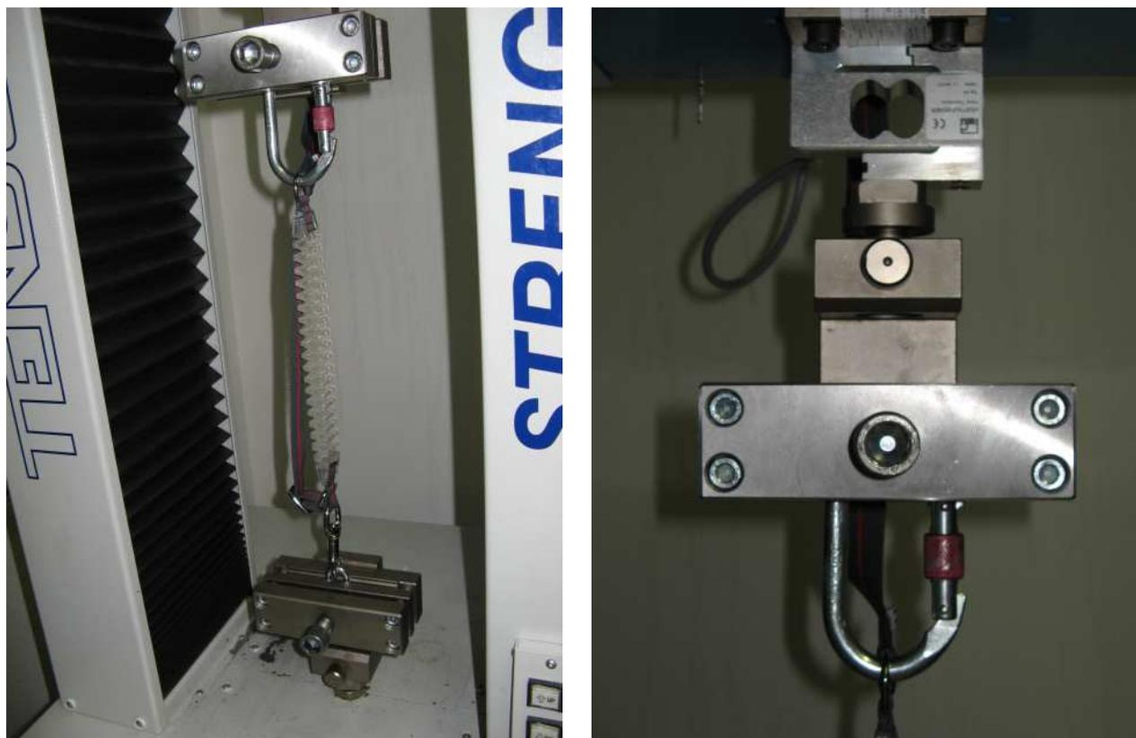
**Picture 1: Static test on leashes; on the right, picture of clamping method and of the load cell 1 kN used to record data of the transmitted force**
