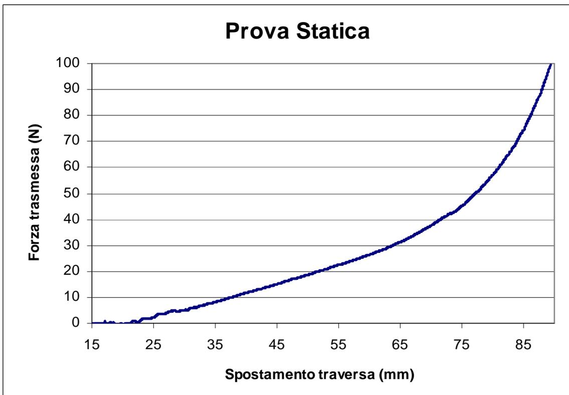
**Picture 2: Path example from a tensile strength test on leash WAW: change of the slope in the final part of the curve is caused by the simultaneous loading of the parallel tape when the accordion is totally elongated**
